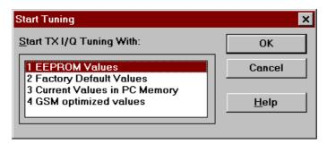
If user selects **4 GSM optimised values**, then tuning is started with values that were saved earlier in GSM band. Note that this selection is available only in PCN mode and when GSM values have been saved to PC memory.
